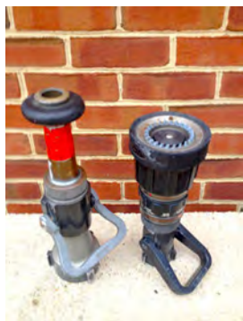
Figure 9.5. On the left is a smooth-bore nozzle that produces a solid stream. On the right is a combination nozzle that can be adjusted from a straight stream to a wide fog stream.
