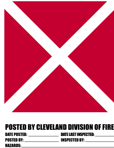
Figure 7.4. A vacancy status sign that warns firefighters that a building is unsafe to enter. Space at the bottom of the sign is for information on specific hazards.
