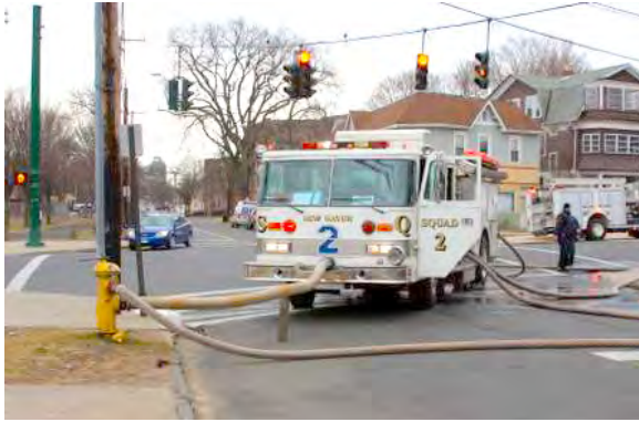
Figure 4.9. A fire hydrant located too close to an intersection can result in pumpers blocking other apparatus access.
